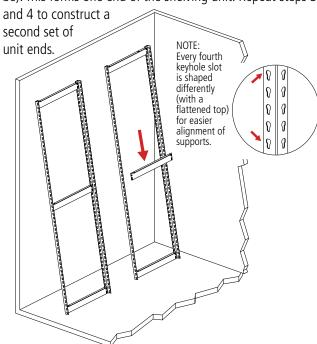
NOTE: If you are planning to install an adder unit, this second set of uprights should consist of ZTP uprights (Ref. No. 2) to act as an intermediate assembly. Carefully review step 2 to better understand.
