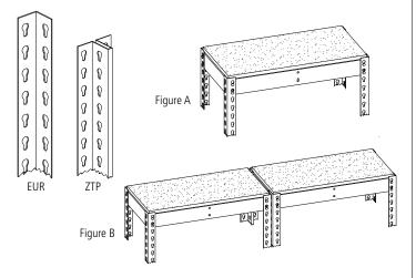
**3.** With the help from an associate, or using a wall for support, connect two EUR uprights (Ref. No. 1) using two front-to-back supports (Ref. No. 3), one at the top and one near the bottom (leaving the bottom-most keyhole slot empty). Be sure the front-to-back supports are fully seated in the keyhole slots as shown.
