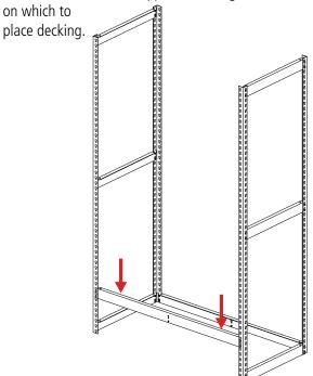
**6.** Attach the remaining shelf supports at the desired shelf levels, making sure that all shelf supports are completely seated in the upright slots.
